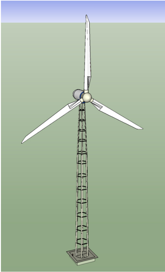
Figure 4.3: A View of the Lattice Tower with Horizontal Bracing
