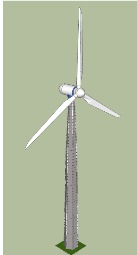
Figure 4.4: A View of the Lattice Tower with Concrete Panel Bracing
