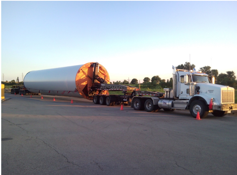
Figure 1.6: Typical Wind Turbine Tower Transportation Configuration
